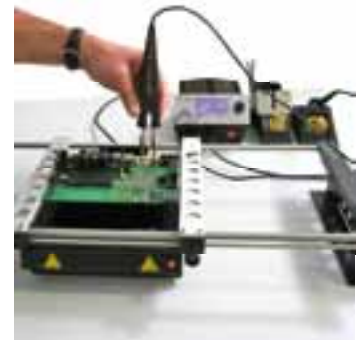
SMD desoldering with the CHIP TOOL desoldering tweezers. Bottom-side preheating with heating plate provides for gentle processes.
